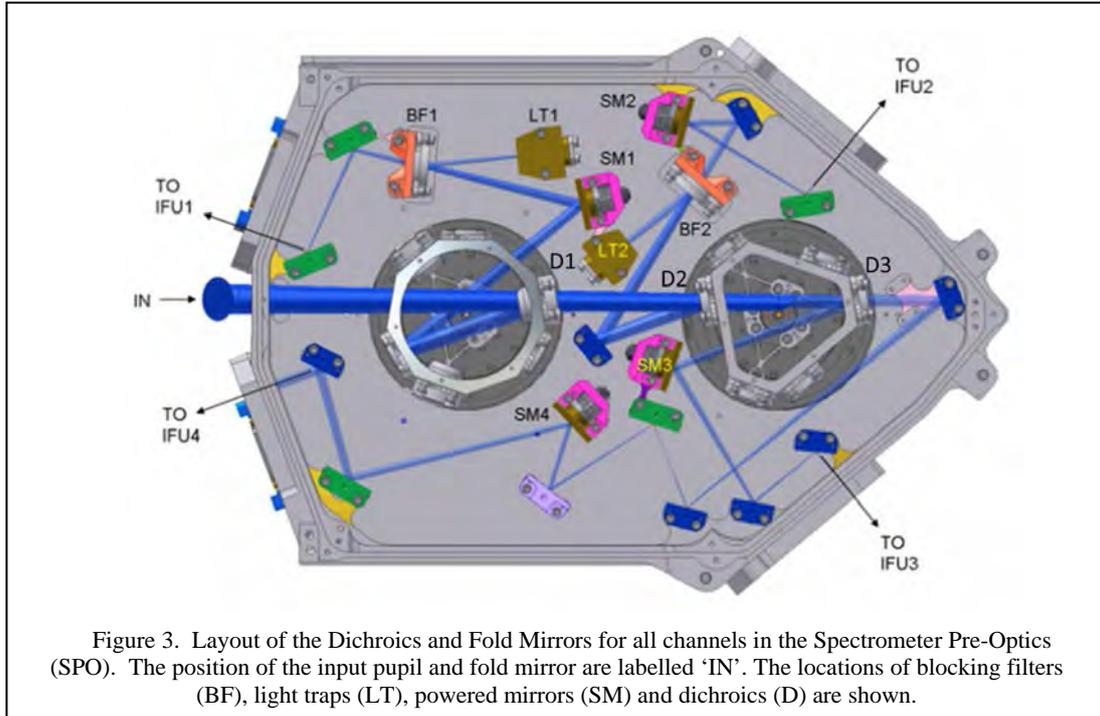
Figure 3. Layout of the Dichroics and Fold Mirrors for all channels in the Spectrometer Pre-Optics (SPO). The position of the input pupil and fold mirror are labelled 'IN'. The locations of blocking filters (BF), light traps (LT), powered mirrors (SM) and dichroics (D) are shown.
