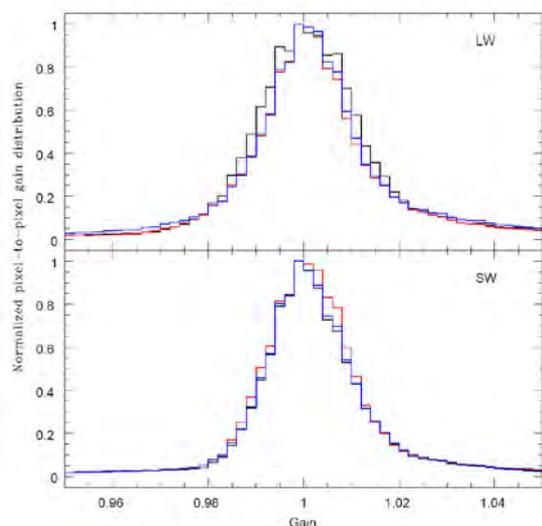
Figure 21. Normalized pixel-to-pixel gain distributions derived from 3 observations for SW and LW detectors (black, red and blue). The FWHMs are 1.91 % and 1.99 % for the SW and LW channels, respectively.
