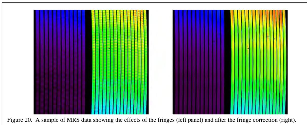
Figure 20. A sample of MRS data showing the effects of the fringes (left panel) and after the fringe correction (right).
