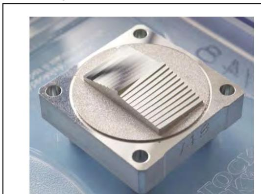
Figure 7. Photograph of the Channel 1 Image Slicer Mirror (Courtesy of Cranfield University).
