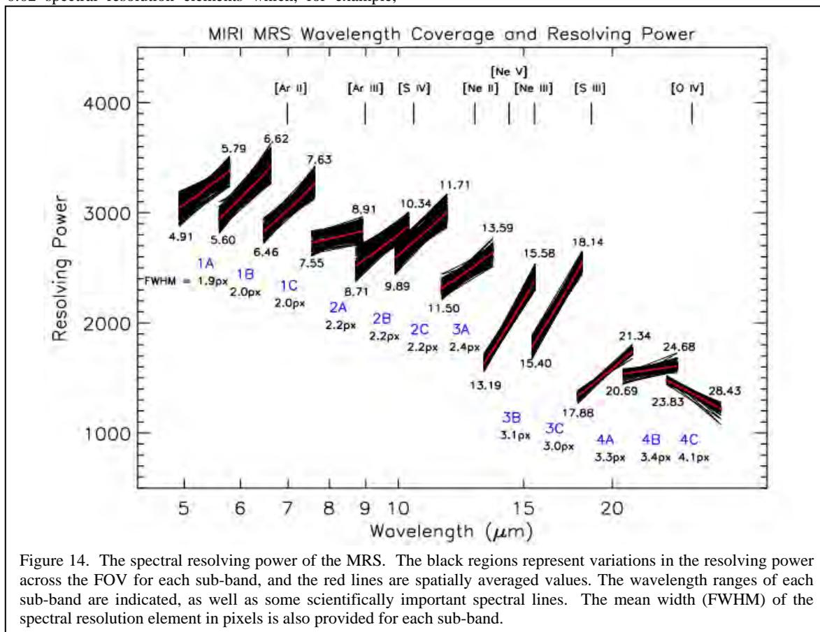
Figure 14. The spectral resolving power of the MRS. The black regions represent variations in the resolving power across the FOV for each sub-band, and the red lines are spatially averaged values. The wavelength ranges of each sub-band are indicated, as well as some scientifically important spectral lines. The mean width (FWHM) of the spectral resolution element in pixels is also provided for each sub-band.
