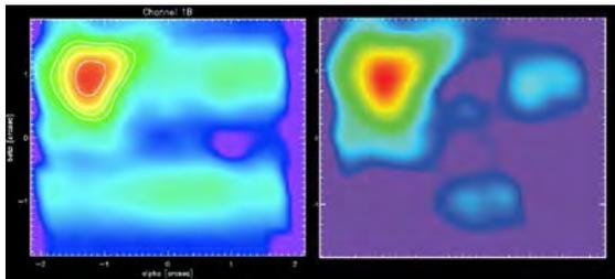
Figure 23. Straylight in Channel 1B. Left: The reconstructed image of a bright, moderately compact source is plotted on a logarithmic scale with contours at 50, 20, 10 and 5 % of the peak signal level. Right: The image after stray-light correction using a proto-type algorithm.
