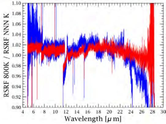
Figure 22. Comparison of the Relative Spectral Response function calculated using observations of the MTS black body at 400 K (blue) and at 600 K (red) with the RSRF at 800 K.
