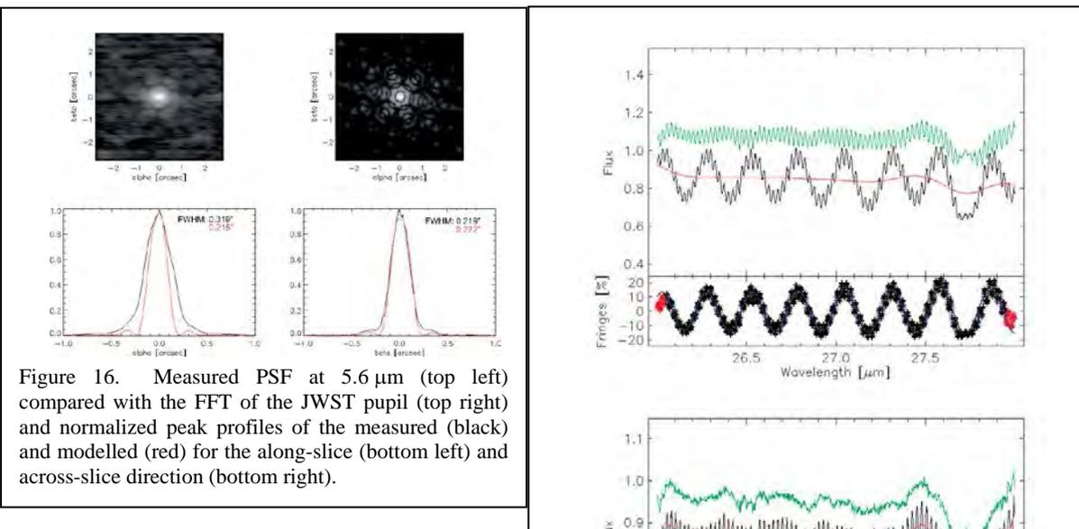
Figure 16. Measured PSF at  $5.6 \mu\text{m}$  (top left) compared with the FFT of the JWST pupil (top right) and normalized peak profiles of the measured (black) and modelled (red) for the along-slice (bottom left) and across-slice direction (bottom right).
