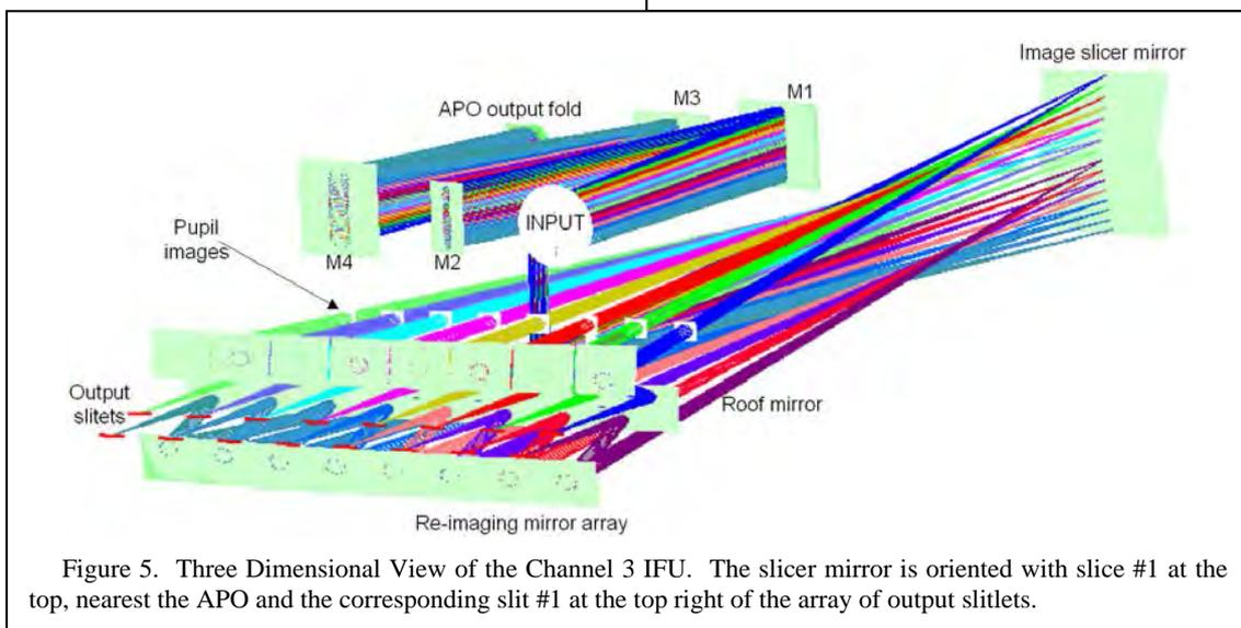
Figure 5. Three Dimensional View of the Channel 3 IFU. The slicer mirror is oriented with slice #1 at the top, nearest the APO and the corresponding slit #1 at the top right of the array of output slitlets.
