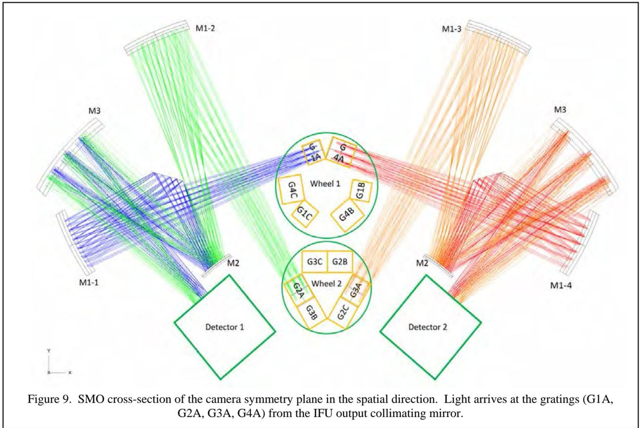
Figure 9. SMO cross-section of the camera symmetry plane in the spatial direction. Light arrives at the gratings (G1A, G2A, G3A, G4A) from the IFU output collimating mirror.
