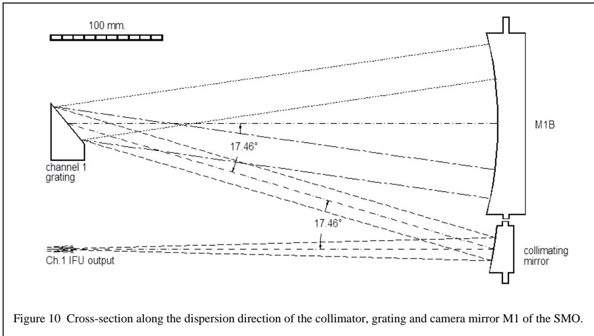
Figure 10 Cross-section along the dispersion direction of the collimator, grating and camera mirror M1 of the SMO.
