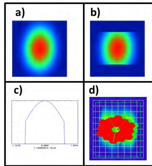
Figure 8. (a) and (b), Input and truncated images on the imager slicer mirror. (c), Cross-section through the peak of the truncated image. (d), Diffraction broadened pupil images (see text for details).
