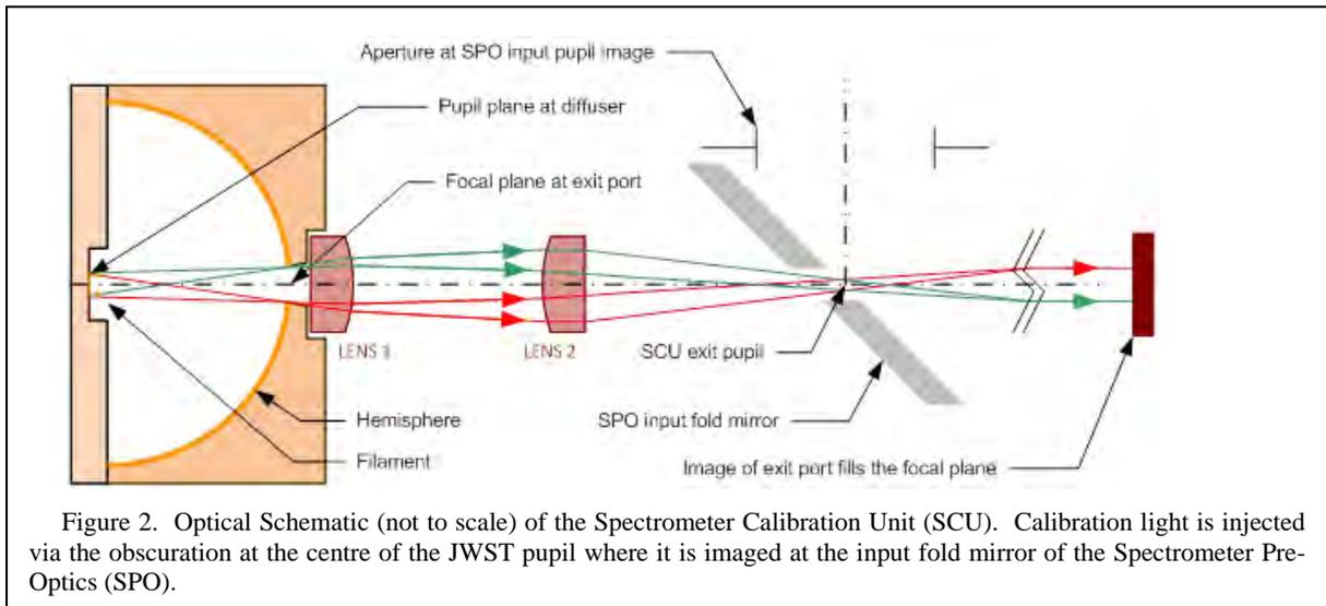
Figure 2. Optical Schematic (not to scale) of the Spectrometer Calibration Unit (SCU). Calibration light is injected via the obscuration at the centre of the JWST pupil where it is imaged at the input fold mirror of the Spectrometer Pre-Optics (SPO).
