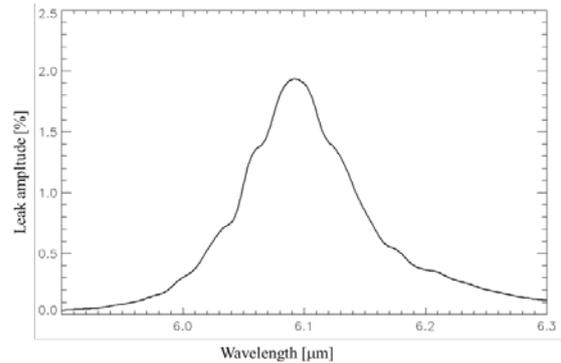
Figure 24. MRS Channel 3A spectral leak profile. This is the fraction of the source spectrum at  $\lambda = 6.1 \mu\text{m}$  which is added to the nominal 12.2  $\mu\text{m}$  spectrum.
