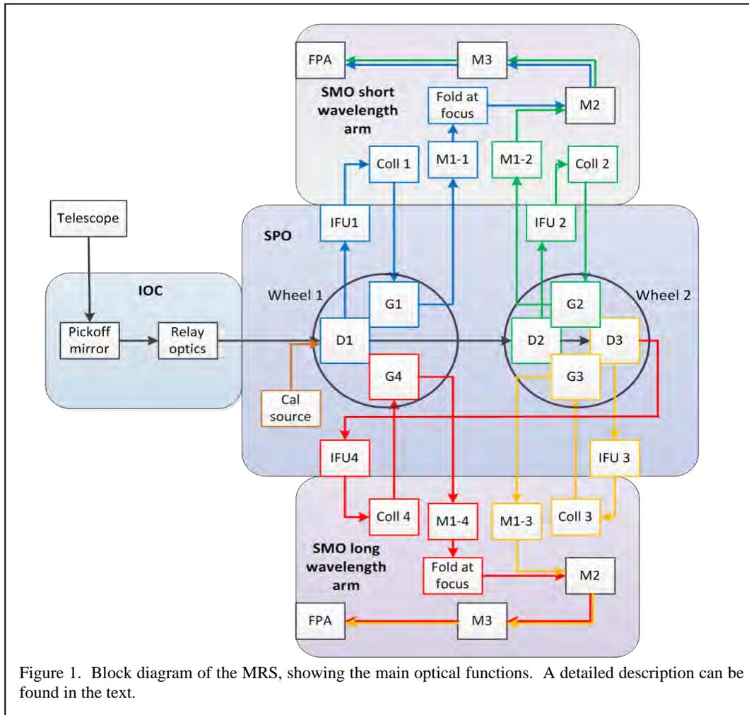
Figure 1. Block diagram of the MRS, showing the main optical functions. A detailed description can be found in the text.
