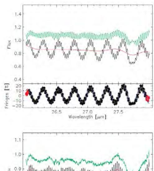
Figure 18. The combined fringes for each channel and sub-band. The data for each neighbouring band are plotted in a different colour for clarity. The main and high frequency fringe components are not resolved on this scale. In Channels 2 and 3 an example of a low frequency beating fringe can clearly be seen. Note: the spectrum is normalized to the peaks of the main fringe amplitude. See text for a description of the solid and dashed-dotted lines.
