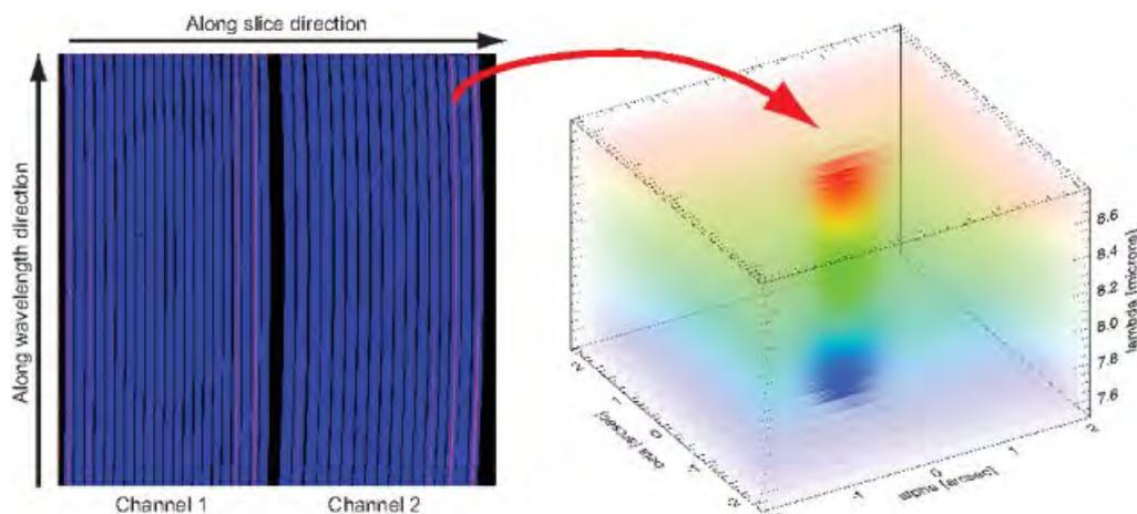
Figure 12. Illustration of the reconstruction process: The detector image for two channels is reconstructed into a 3D cube with two spatial dimensions ( $\alpha$  along the slice and  $\beta$  across the slice) and one spectral dimension ( $\lambda$ ).
